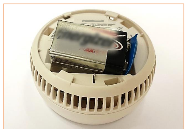
External battery which requires annual replacement
